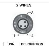
This module is fitted with two M8 3 pin female connectors.
